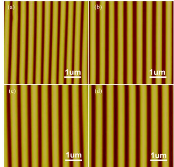
Fig. 2. AFM images of PDMS templates with different periods fabricated by different duration of the oxygen plasma treatment. (a) 2 min; (b) 3 min; (c) 4 min; (d) 5 min.
