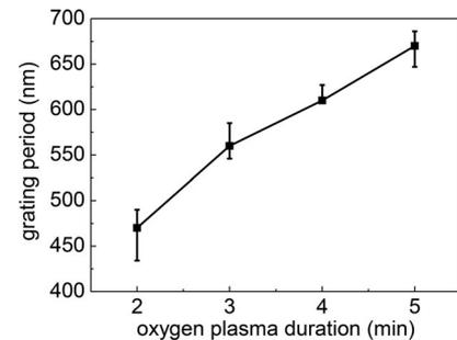
Fig. 3. Error bar plot of periods of PDMS gratings fabricated by different durations of oxygen plasma treatment. The black squares show the average values of the grating periods.
