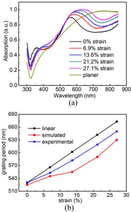
Fig. 6. (a) Absorption spectra of metallic gratings fabricated with "restretching step" at different external strain. (b) The relationship between grating periods and external strain values.
