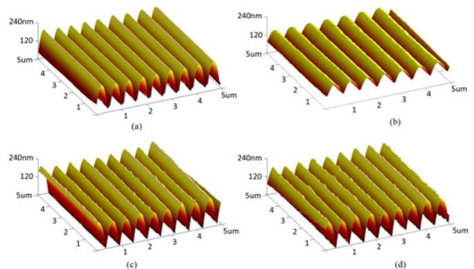
Fig. 4. AFM images of the PDMS template with an amplitude of (a) 150 nm and period of 560 nm, (b) restretching the PDMS template with a strain of 30% and coating Ag film, and (c) releasing the second tension. (d) AFM image of the metallic gratings after 30 stretching-releasing cycles.
