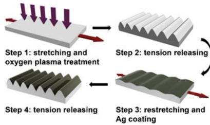
Fig. 1. Schematic illustration of procedures used to fabricate stretchable metal gratings: step 1, stretching the PDMS sheet and oxygen plasma treatment; step 2, releasing the pretension to form ordered wrinkles template; step 3, restretching the wrinkles template and coating Ag film; step 4, releasing the second tension to finish the metallic gratings fabrication.
