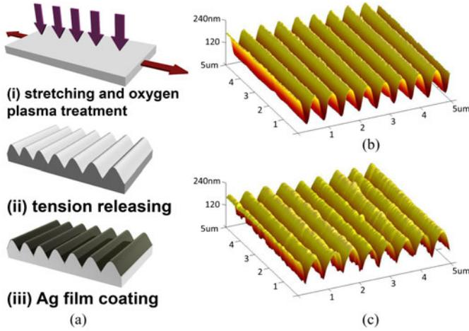
Fig. 5. (a) Fabrication procedure of the stretchable metallic gratings without the restretching step. AFM images of the metallic gratings fabricated (b) without the restretching step and (c) after 30 stretching-releasing cycles.
