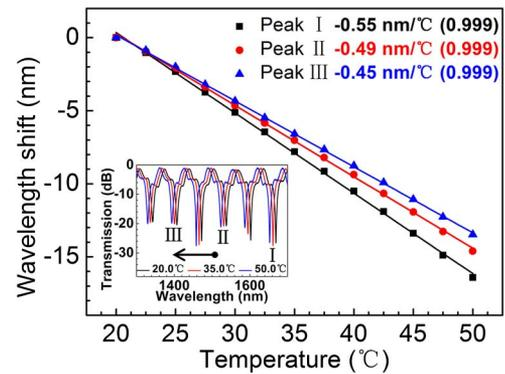
Fig. 5. (Color online) Relationships between temperature and wavelength shift of different resonant peaks for the air-sealed OMT. The inset shows the typical transmission spectrum under different temperature.
