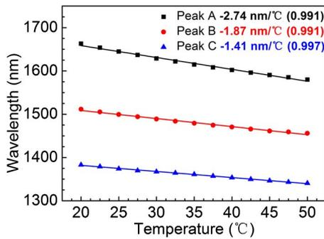
Fig. 4. (Color online) Simulation results of TSCs from thermo-optic effect of isopropanol for different resonant peaks.
