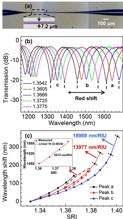
Fig. 2. (Color online) (a) Optical microscope image of the OMT. (b) Typical transmission spectrum of the unsealed OMT under different RI solutions. (c) Wavelength shift of the resonant peaks with different RI solutions. The inset shows the linear fitting result of peak  $b$  in the RI range of 1.3605–1.3775.
