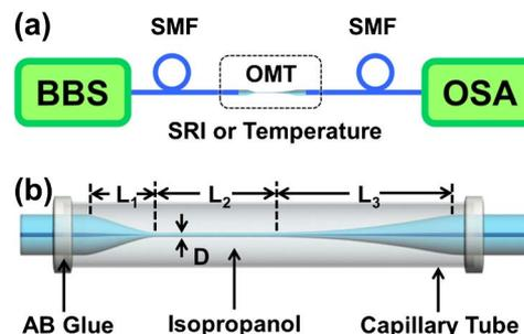
Fig. 1. (Color online) (a) Experimental setup for sensing measurement. (b) Schematic diagram of the isopropanol-sealed OMT in a capillary.
