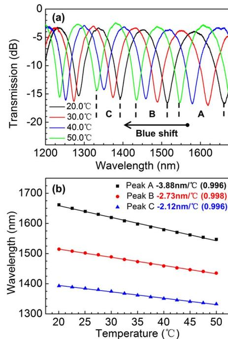
Fig. 3. (Color online) (a) Typical transmission spectrum of the isopropanol-sealed OMT under different temperatures. (b) Relationships between temperature and wavelength of different resonant peaks. The numbers in brackets represent Adj.  $R$ -Square.
