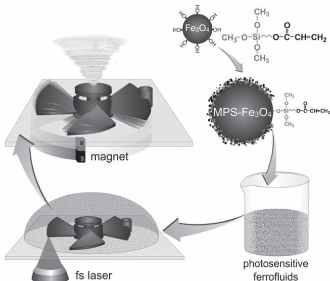
**Scheme 1.** Fabricative procedures of remotely controllable micro-nanomachines.
