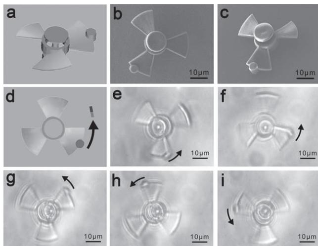
**Figure 4.** Remote control of the micro-turbine in acetone. a, model of the micro-turbine. b,c) SEM images of the micro-turbine. d) top view schematic model for circumgyration. e–i) optical microscopy images of the micro-turbine in a circumgyration cycle. For remote control and observation of the micro-turbine, a piece of ferromagnet was placed on a vortical device around the objective lens (Figure S1).
