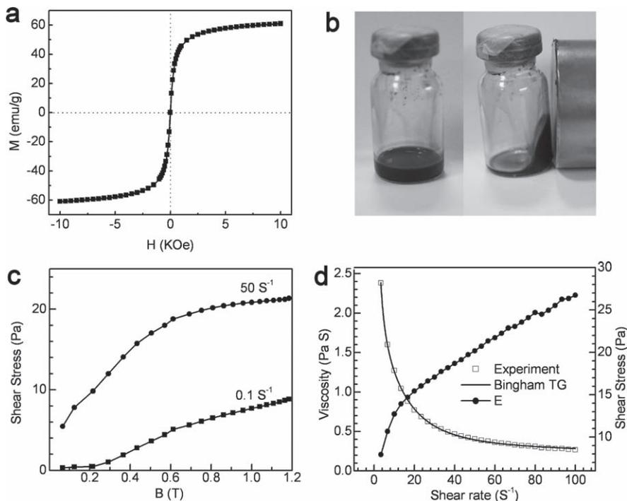
**Figure 2.** a) VSM spectrum of the MPS-Fe<sub>3</sub>O<sub>4</sub>. b) Photographs of static ferrofluid and the ferrofluid under magnetic force. c) Shear stress curves of the ferrofluid as a function of magnetic field intensity at the shear rate of 0.1 S<sup>-1</sup> and 50 S<sup>-1</sup>. d) Viscosity and shear stress curves of the ferrofluid as a function of the shear rate under the magnetic field intensity of 0.43 T.
