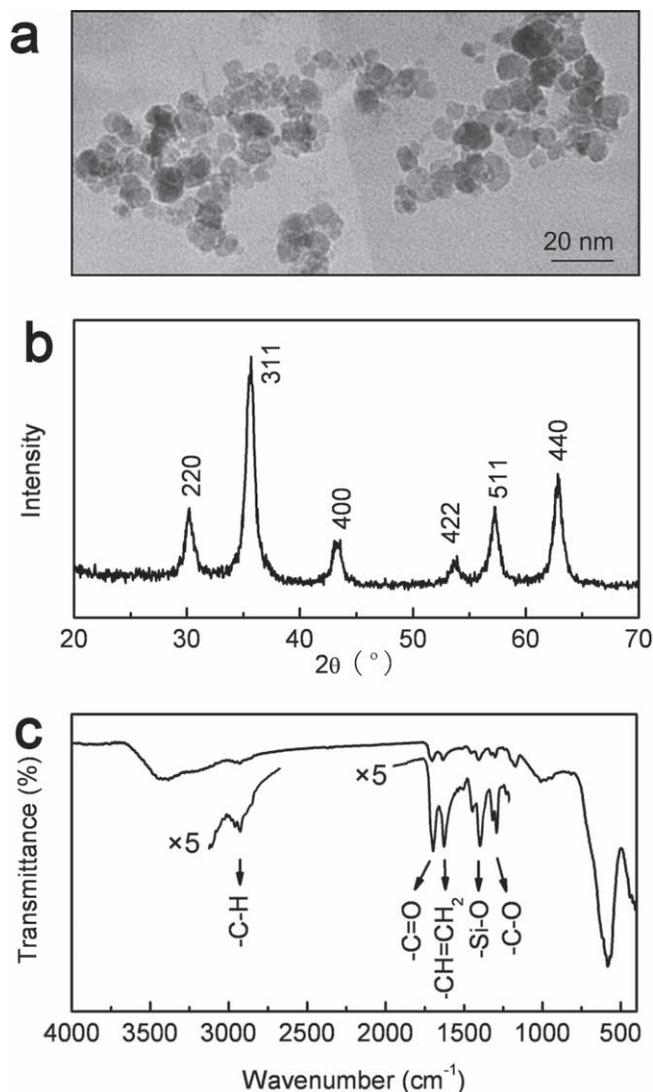
**Figure 1.** Characterizations of MPS-Fe<sub>3</sub>O<sub>4</sub> nanoparticles. a) TEM image of MPS-Fe<sub>3</sub>O<sub>4</sub> nanoparticles. b) XRD pattern of MPS-Fe<sub>3</sub>O<sub>4</sub> nanoparticles. c) FT-IR spectrum of MPS-Fe<sub>3</sub>O<sub>4</sub> nanoparticles.
